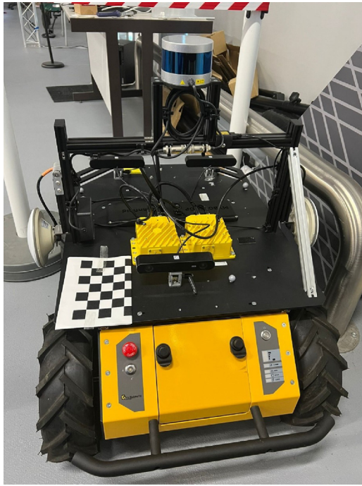
Fig. 3. Husky A200 vehicle platform (centre for autonomous & cyber-physical systems, Ground autonomy Lab, Cranfield University).
