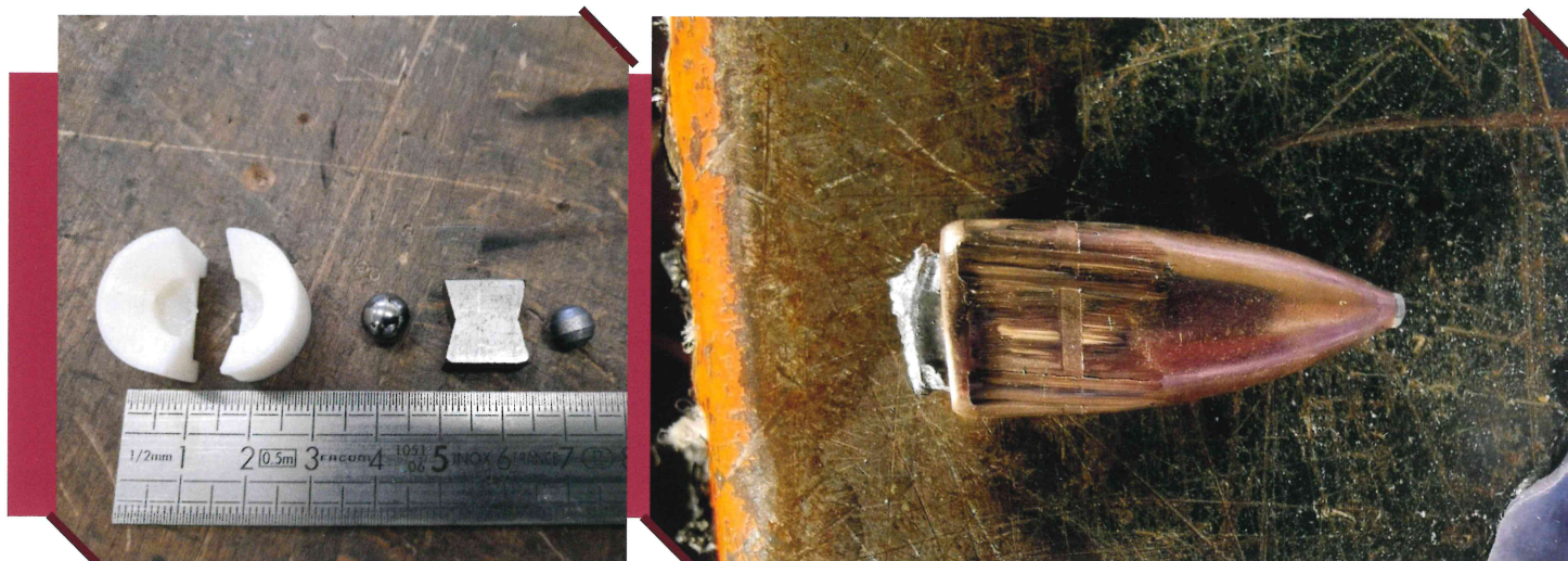
Figure 2: Left - Images of the three gas-gun projectiles, plastic sabot, and Right - rifle-range projectile (7.62 NATO steel cored ball round, post impact)
