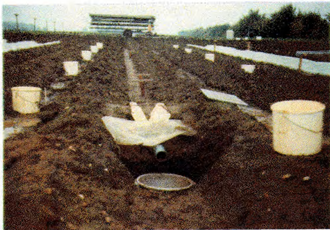
Figure 6.6 Discharge measuring devices in the field
