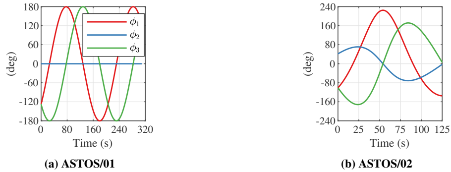
Fig. 14 Simulated relative attitude states for the ASTOS dataset of the target frame with respect to the chaser frame.
