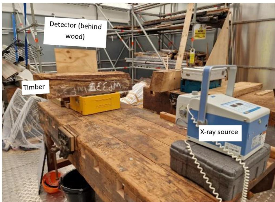
Figure 62: Radiography set up in shipwright working area. Image courtesy Dr Mark Viner, annotations by author
