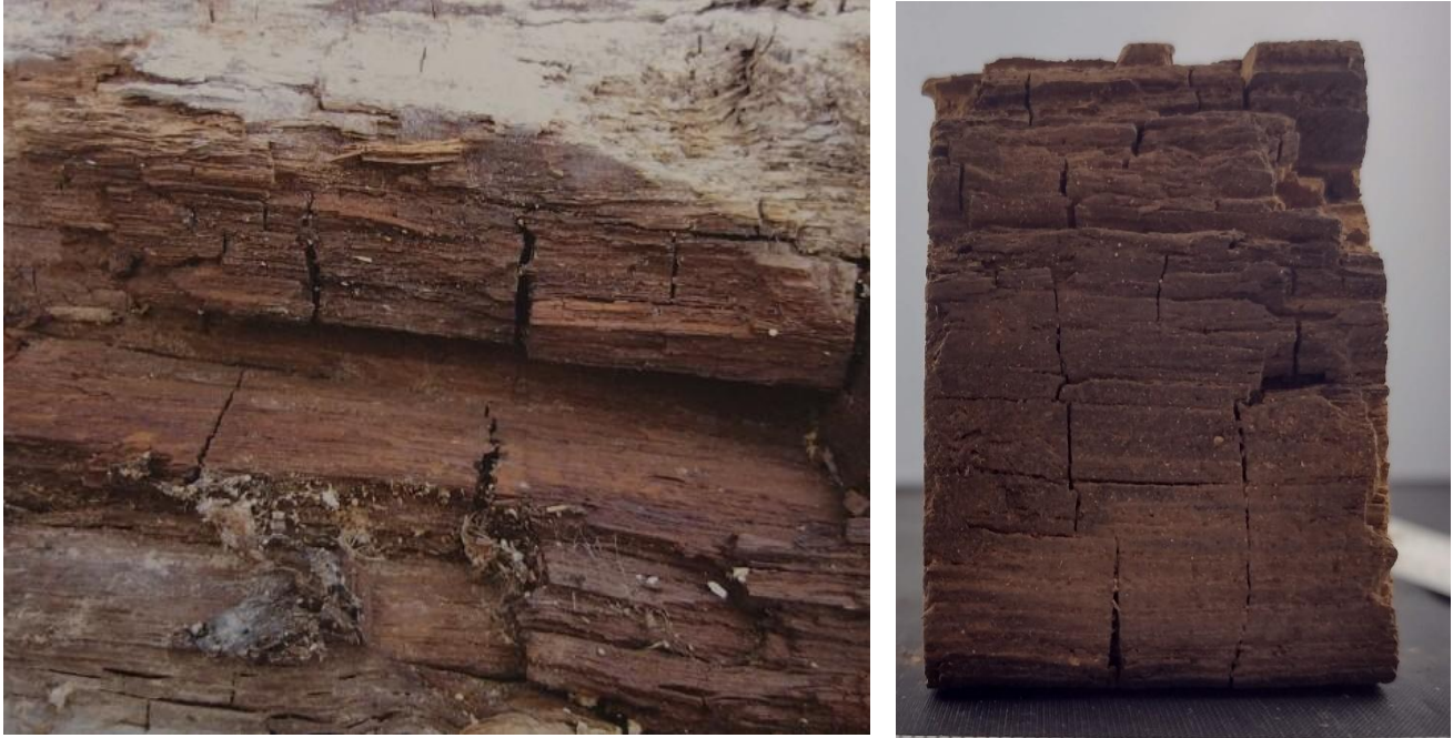
Fig C2(a) and (b): (a- left) Characteristic brown rot cubical fractures on timber from McCaig and Ridout 2012: 186. (b- right) Brown rot cubical fractures on sample A1A
