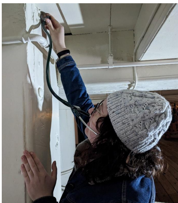
Figure 60: Testing a stethoscope on areas of suspected larval activity next to a fresh-looking exit hole on the timber connecting the bowsprit to the ship. Image courtesy Dr Fiona Brock
