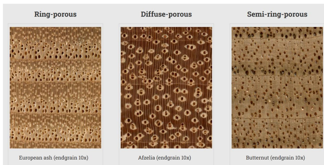
Figure 19: Different porosity types found in hardwoods. Image from Meier 2023b
