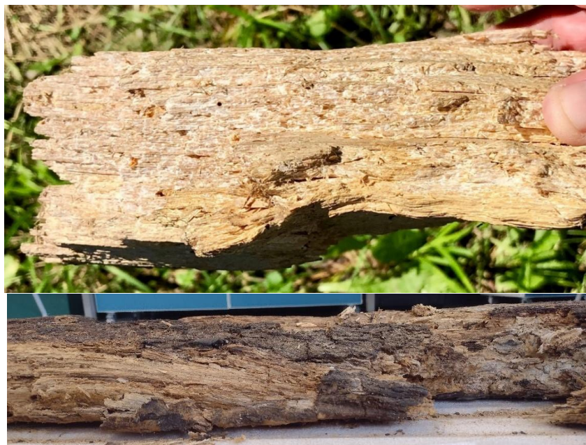
Fig C3(a) and (b): (a- above) Characteristic white rot decay on timber. The timber is spongy and lightweight, and often 'stringy'. From Goodell et al 2020: 8. (b-below) White rot fungus on the plank prior to cutting
