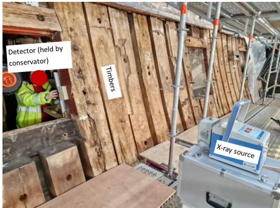
Figure 63: Radiography set up for in situ timbers. Image courtesy Dr Mark Viner, annotations by author
