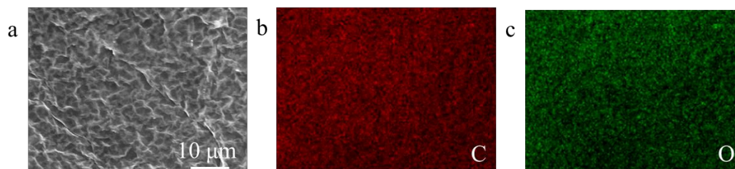
Figure S3. Surface elemental mapping images of the GO membrane surface. (a) Surface SEM image of the GO membrane. (b) Elemental mapping of carbon (C) on the GO membrane. (c) Elemental mapping of oxygen (O) on the GO membrane.
