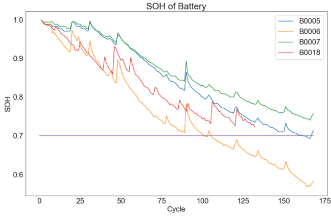
Fig. 1. The relationship of SOH and Cycle for four Li-ion batteries (# 5, 6, 7 and 18).
