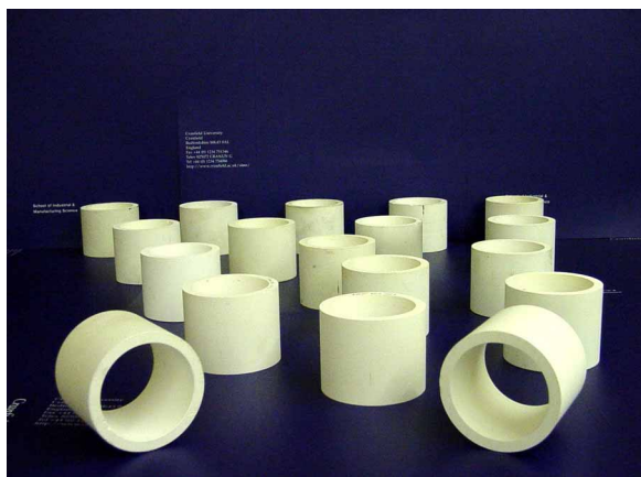
Fig. 1 Porous ceramic hydrostatic journal bearings produced by the SC technique [6]
