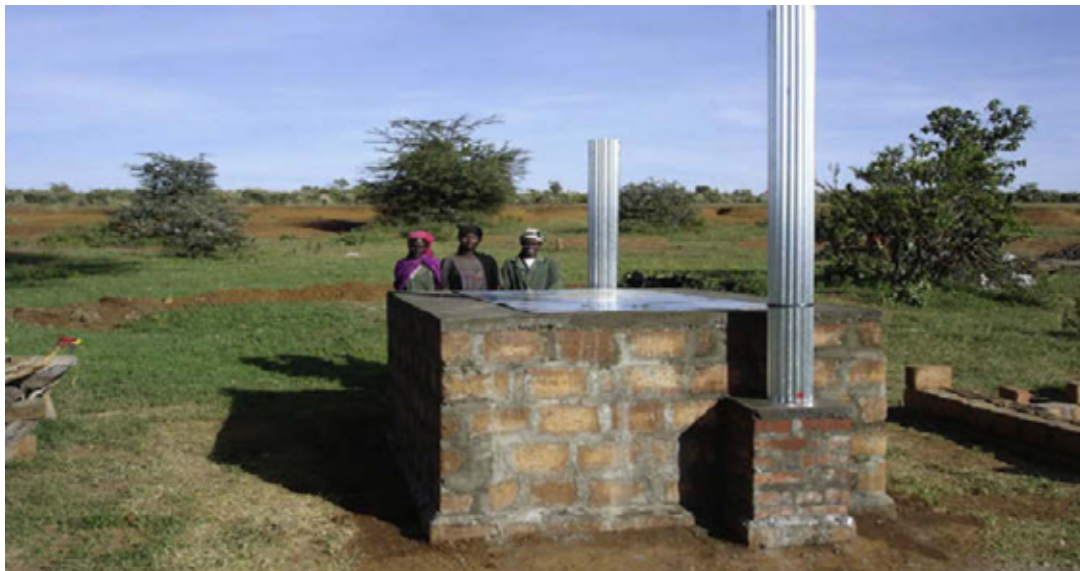
Figure 2 - 8: Adam-retort charcoal kiln type built in Rift valley, Kenya (Adam, 2009).
