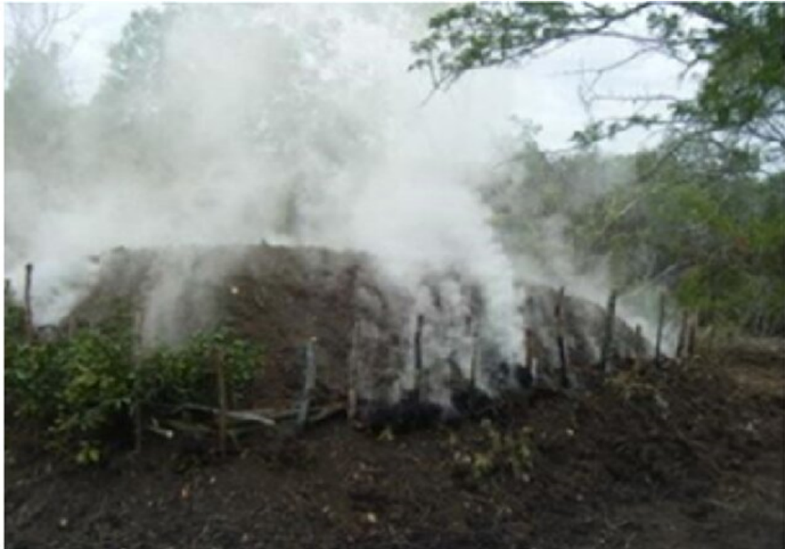
Figure 2 - 6: Image of traditional earth kiln showing charcoal production in Tanzania (Msuya, 2011).
