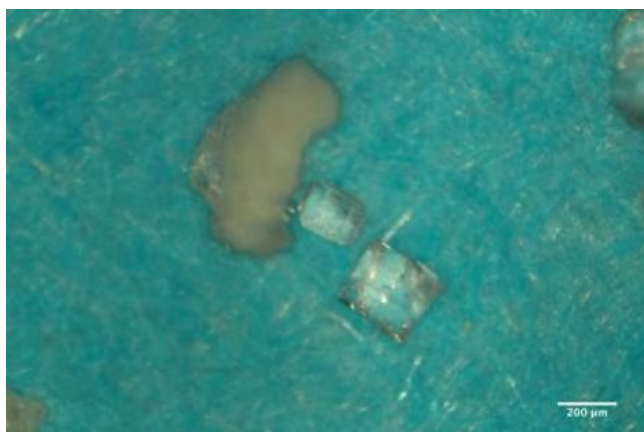
Figure 4. Optical images of inert moulding powder sieve fractions (left) < 0.425 mm fraction with uncoated filler and (right) < 0.425 mm fraction with a well-coated agglomerate example. LabRAM acceleration at 25 G during addition of anti-solvent (IPA) at 6 cm 3 min -1 . See supplementary data for more details.
