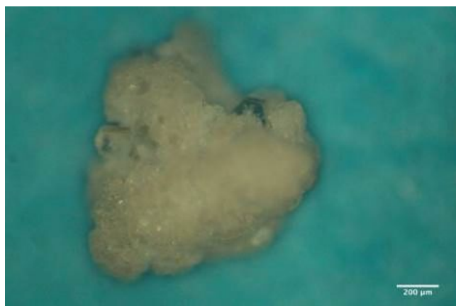
Figure 4. Optical images of inert moulding powder sieve fractions (left) < 0.425 mm fraction with uncoated filler and (right) < 0.425 mm fraction with a well-coated agglomerate example. LabRAM acceleration at 25 G during addition of anti-solvent (IPA) at 6 cm 3 min -1 . See supplementary data for more details.
