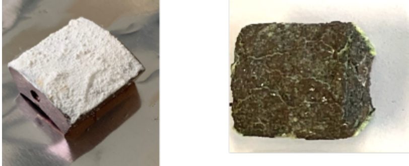
Figure 3-5: Deposit coated sample before and after 1000 hours exposure
