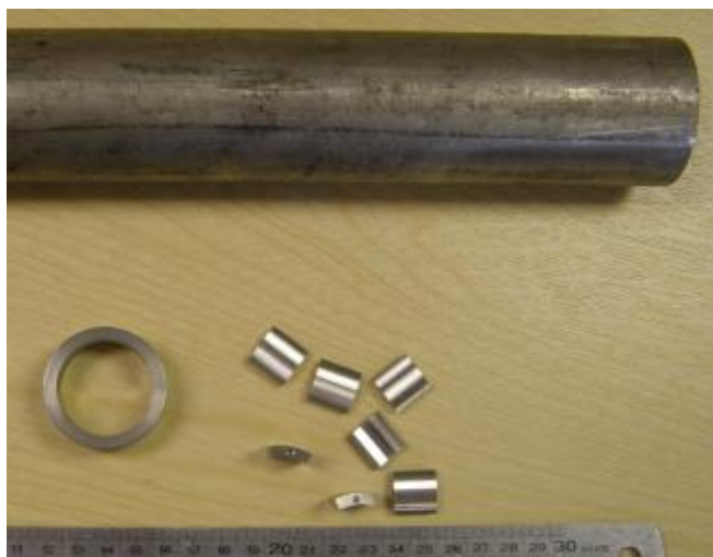
Figure 3-2: An alloy tube, ring, and curved samples [111]
