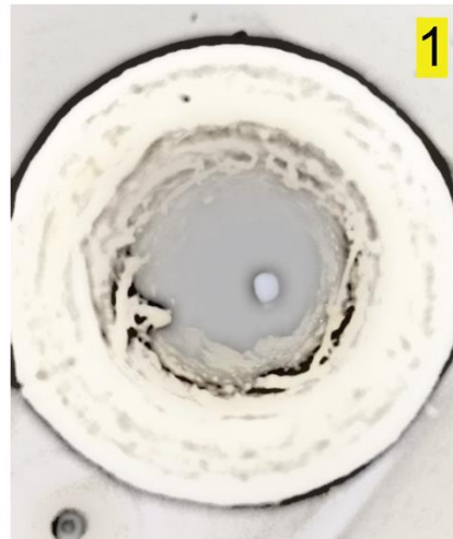
Filter after first evacuation
