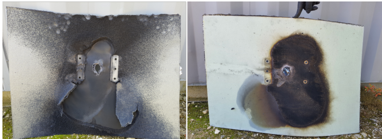
(c) Post test material D: Hot face (left) and Cold face (right)
