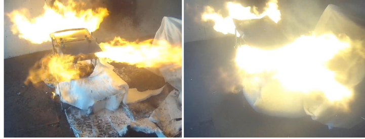
Fig. A3: No burn through of test substrate facing cell ejecta of two 86Ah cells
