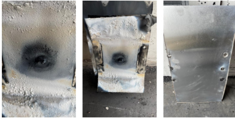
(a) Post test material E: Hot face(left and center), Unaffected cold face (right)
