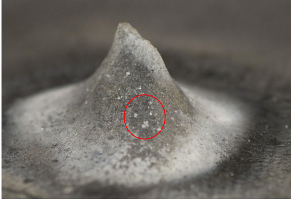
Fig. 21: Hot particle attachment on ablative material
