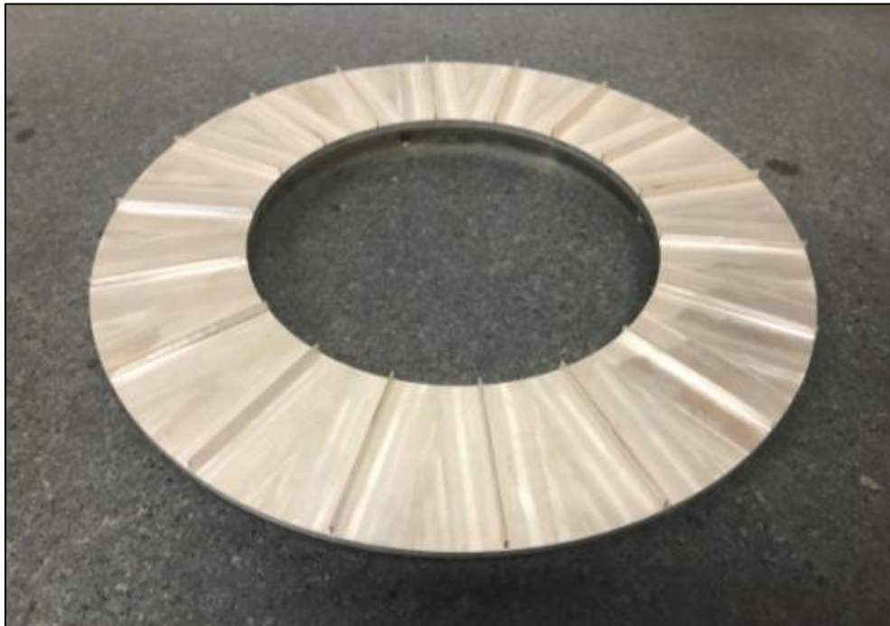
Figure 4-4 Shear ring used in bevameter (NATO NRMM CDT (2018))
