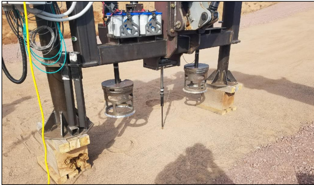
Figure 4-6 Cone penetrometer test (NATO NRMM CDT (2018))
