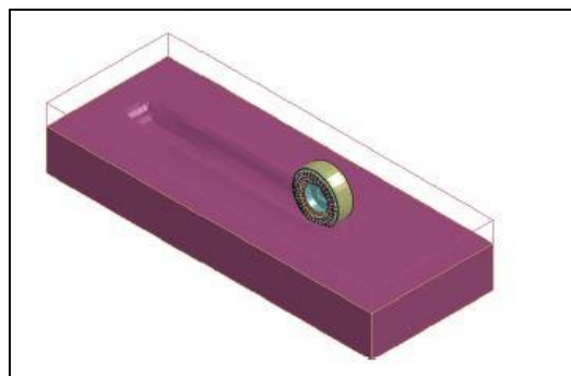
Figure 2-17 Overview of tyre / soil interaction model using FEM in LS-DYNA (Wright (2012))
