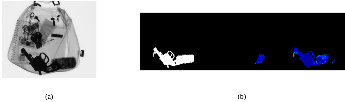
Figure 7. (a) Single-energy X-ray imagery of a bag (b) weapon cluster disjoint (X-ray image from 18 )
