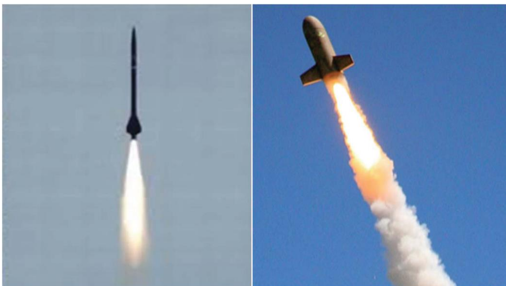
Figure 2: Burn trails of smokeless (left) and perchlorate (right) propellants [17]
