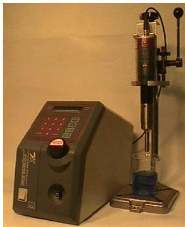
Figure 48: Heat Systems XL2020 sonicator, fitted with a 1/2" probe.
