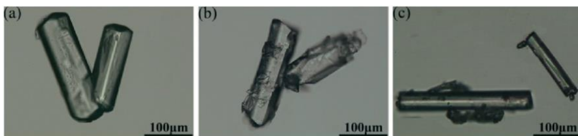
Figure 23: Optical micrographs of AP/crown ether cocrystals (a) AP/18C6, (b) AP/B18C6 and (c) AP/DB18C6 [104]
