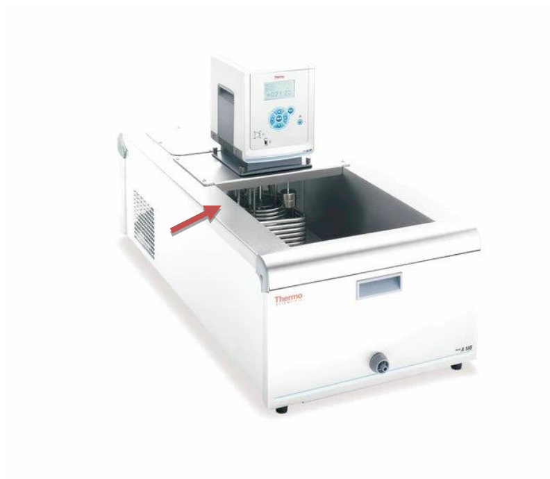
Figure 42: ThermoFisher Scientific Haake A 10B water bath fitted with AC200 immersion circulator.
