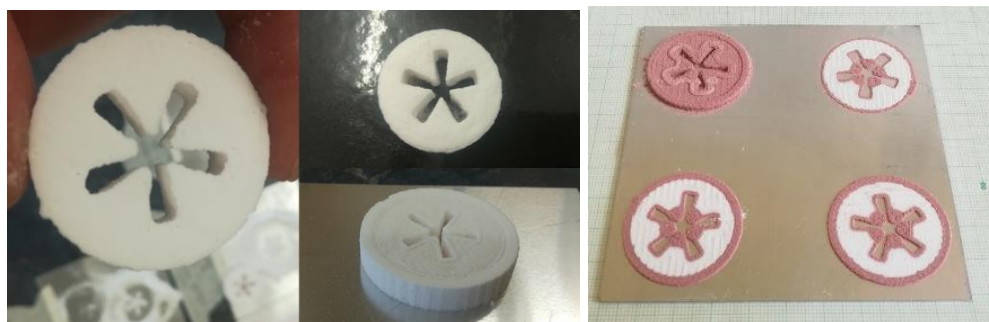
Figure 10: Propellant grains manufactured using the selective powder deposition system at Cranfield, showing complex port geometries and deliberate composition variation [47]
