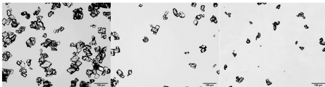
Figure 56: 10g magnetic stirrer bar crystallisations at 400, 800 and 1200 RPM (left-right) showed a tendency towards smaller particle sizes, increased opacity, and extensive secondary nucleation at higher agitation rates. Scale 100 µm.
