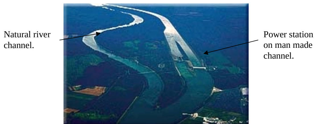
Figure A3.2 Image demonstrates the layout of a river retention scheme (Integrated Rhine Programme website, 2003)
