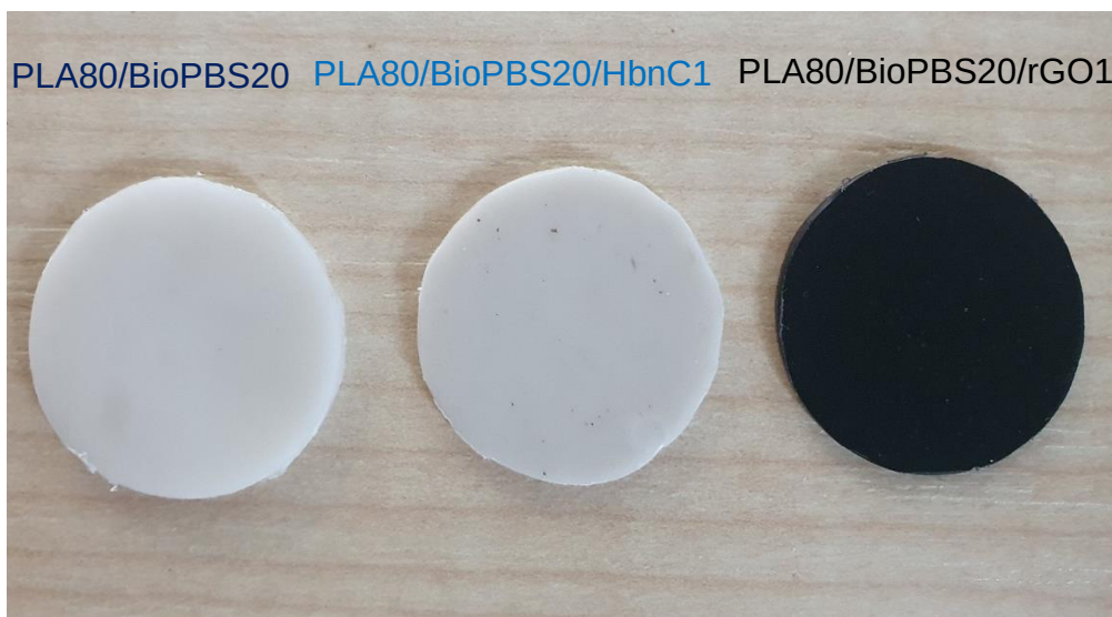
Figure 3-8 As-fabricated cylindrical plates for use in the rheological characterisation of designated filament material formulations
