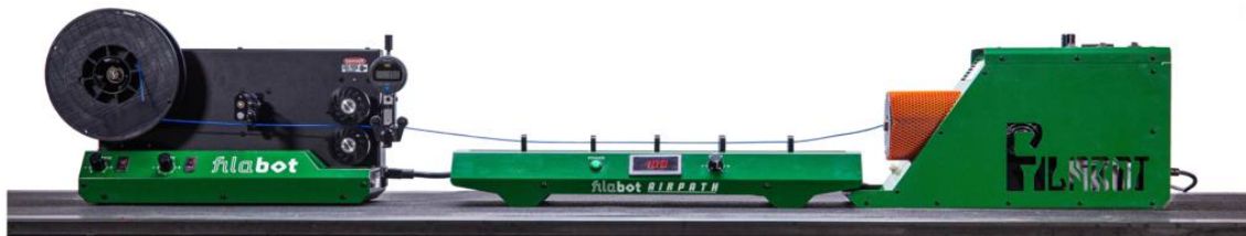
Figure 3-1 Filabot EX2 equipped with a set of cooling fans, diameter measuring device, and filament winder and spooling unit.
