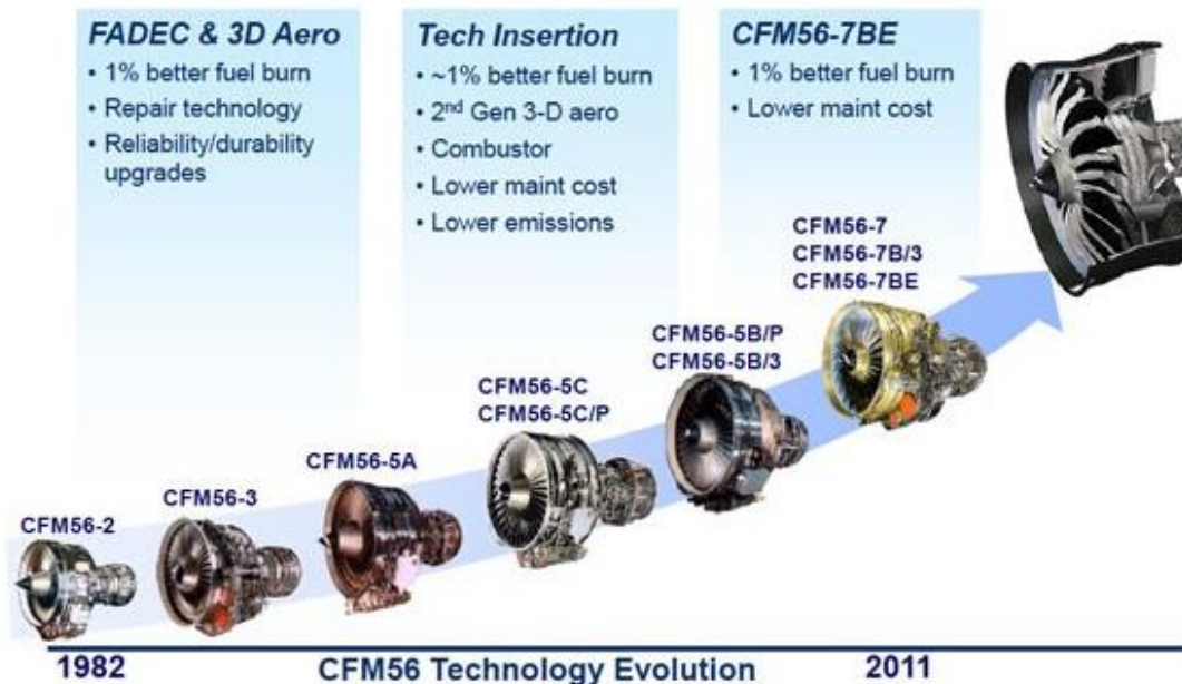
Figure 2-6: CFM56 Engine Evolution
