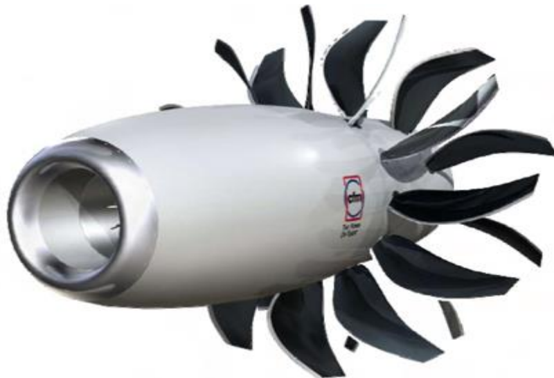
Figure 2-18: Open Rotor Concept [52]
