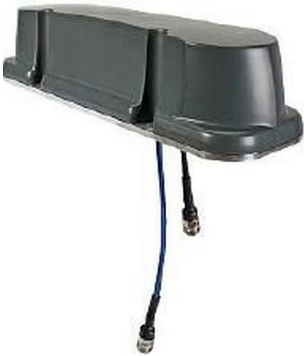
FIGURE 11. Huber+Suhner SENCITY Rail MIMO antenna technical specifications deployed in operational validation. The antenna covers 694-4900 MHz with a 4×4 MIMO configuration, weighs 1.5 kg, and has an IP67 weatherproof rating. Roof mounting provided optimal line-of-sight for both terrestrial cellular and LEO satellite connectivity. Technical specifications validated through manufacturer datasheets and field performance measurements.
