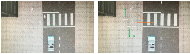
FIGURE 3. Honda Civic pedestrian crossing validation scenario. Top: Reactive baseline control maintains constant velocity until pedestrian detection. Bottom: APACC predictive response with early deceleration initiated 1.8 s before baseline, enabled by the symbolic layer's pedestrian intent inference. Vehicle dynamics parameters provided by Honda Motor Europe ensure simulation fidelity.
