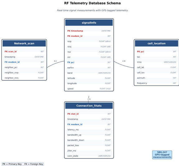
FIGURE 10. Database schema for real-time RF telemetry collection showing relationships between signal measurements (signalInfo), network scanning results (Network_scan), cell tower identification (cell_location), and connection performance statistics (Connection_Stats). This structured data model enabled efficient LSTM training and real-time prediction during operational deployment.
