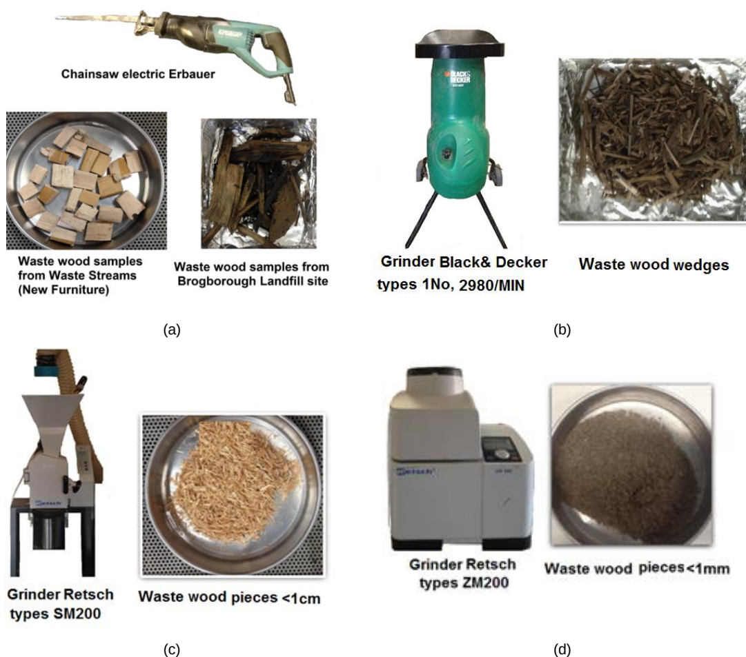
Figure 5-3. Grinding of waste wood samples.
