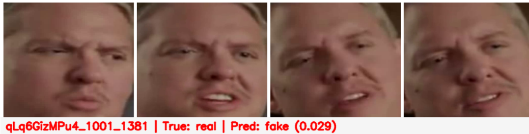
Fig. 9. False Positive – Real video (qLq6GizMPu4_1001_1381) misclassified as fake (confidence 0.029). Compression and motion artifacts mimicked deepfake traces.
