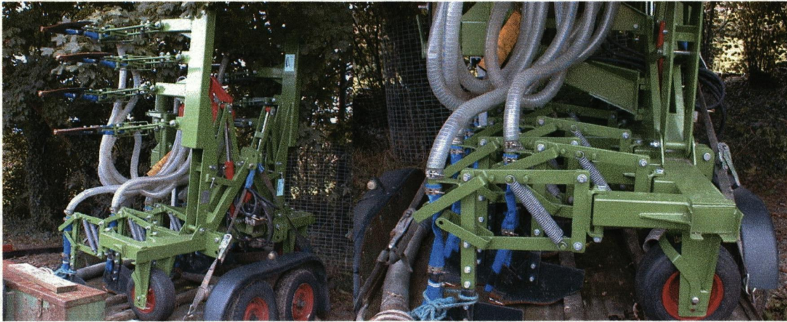
Fig. 12.1. The production model based on the development of the 40WNDLi injector tine; known as the “Greentrac Growing Crop Injector”.
