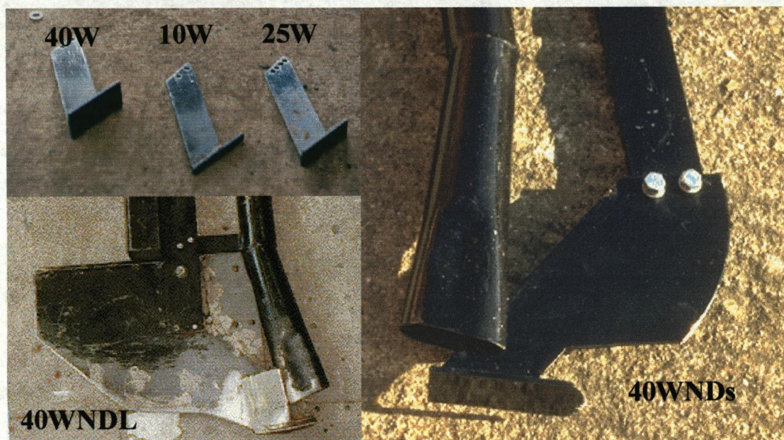
Fig. 2.2. Prototype single-piece injector tines.
