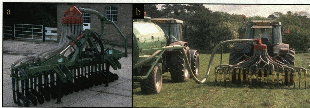
Fig. 4.2. a) slipper foot injector & b) tanker and umbilical supply for plot applications.
