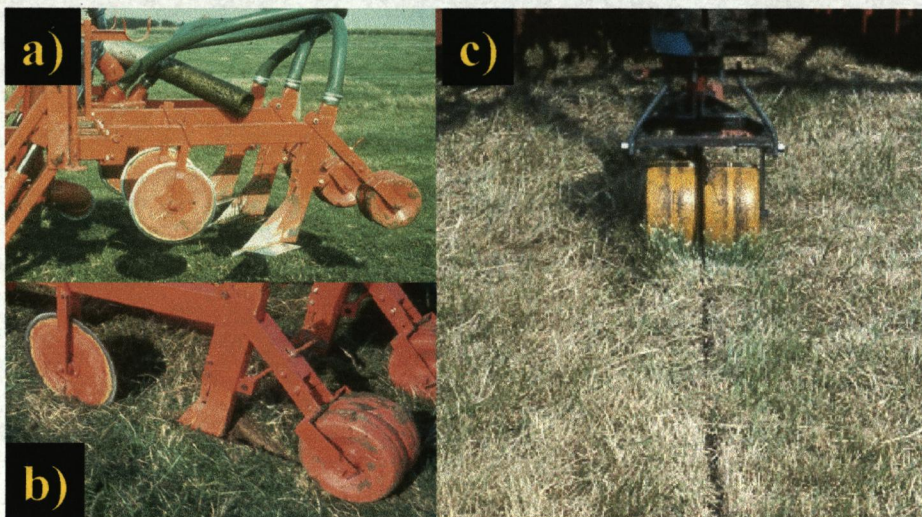
Fig. 1.3. Deep injector design; a) & b) prototype injector and c) press-wheel trials.
