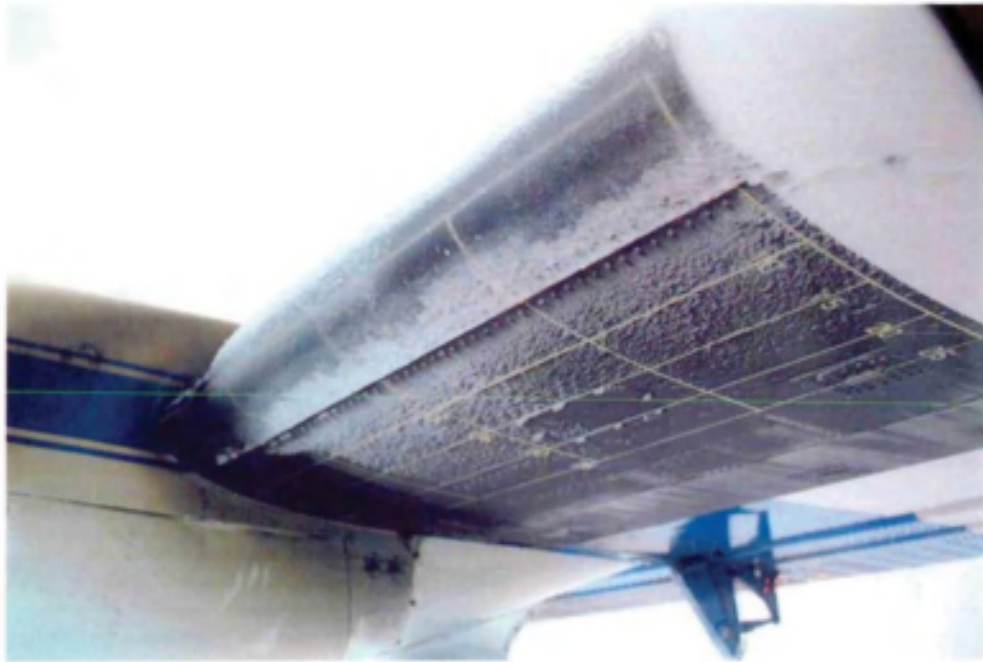
Figure 1: Ice Accretion On Wing Leading Edge (OHC Twin Otter) 1
