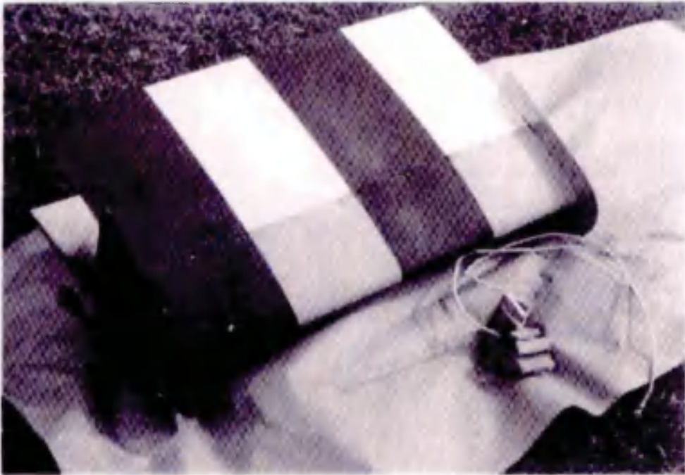
Figure 17: Lear fan Leading Edge & EIDI Bumper Coil. Source: Paramasivam & Zumwalt 23
