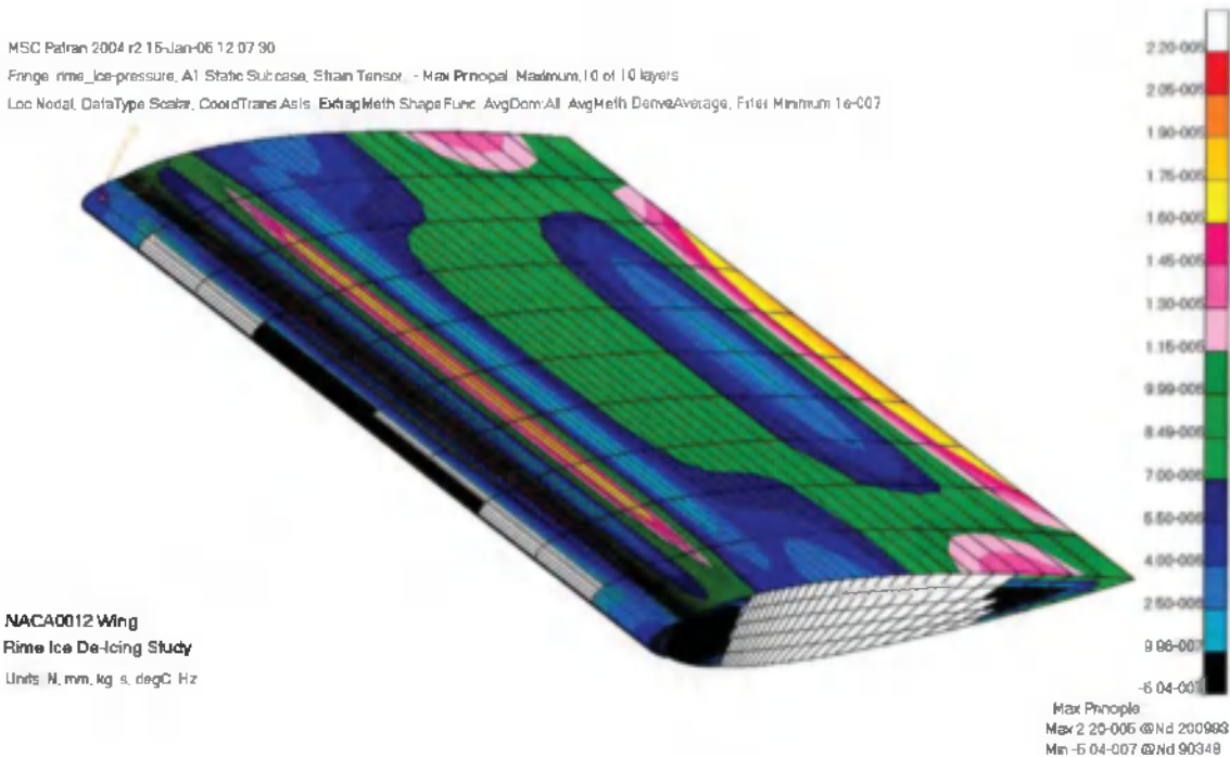
Figure 50: Strains In The Rime Ice Contaminated Wing Subject To Aerodynamic Pressure
