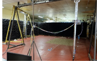
Figure 1. The GBSAR laboratory in a bistatic configuration, measuring a gravel scene.
