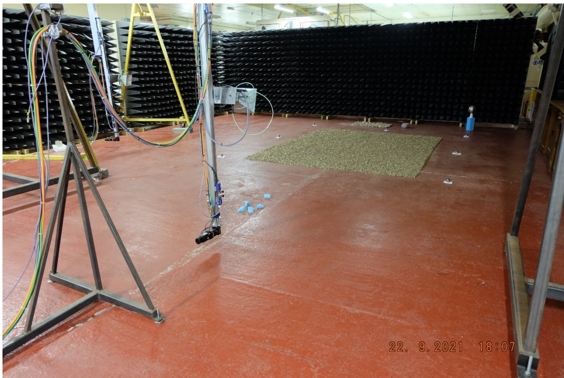
Figure 3.1 Image showing the GBSAR laboratory and scanning system with a gravel scene.
