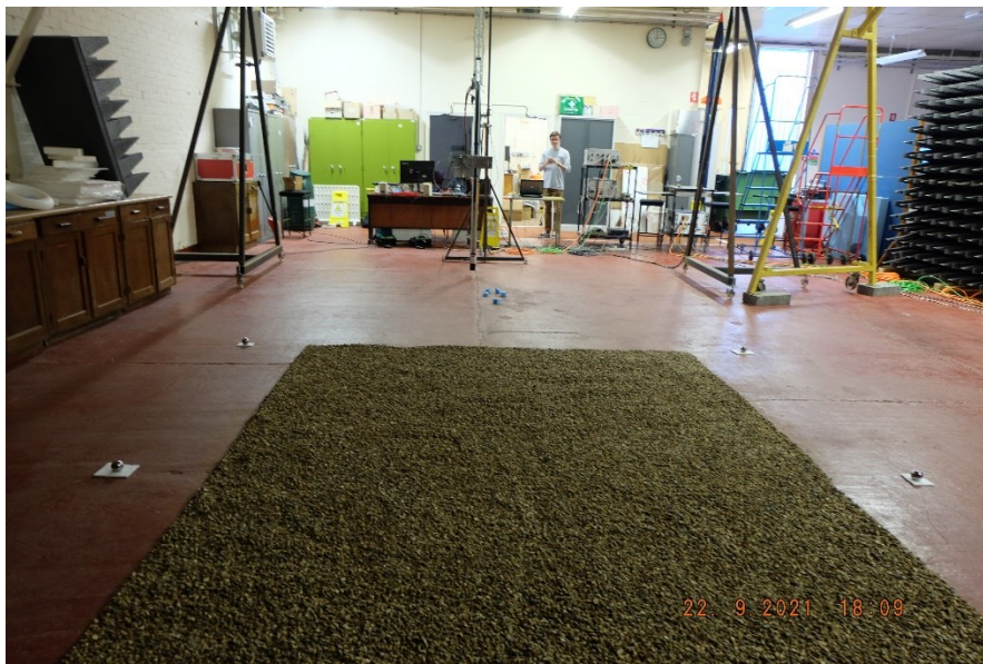
Figure 3.5 Photograph of large rectangular gravel region which was aligned with the transmitter (brown) rail. The receiver was mounted on the yellow rail.
