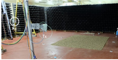
Figure 2. The GBSAR laboratory in a bistatic configuration, measuring a gravel scene. The locations of the transmitter (Tx) and receiver (Rx) are marked. Several metal spheres are positioned around the gravel to aid alignment checks.
