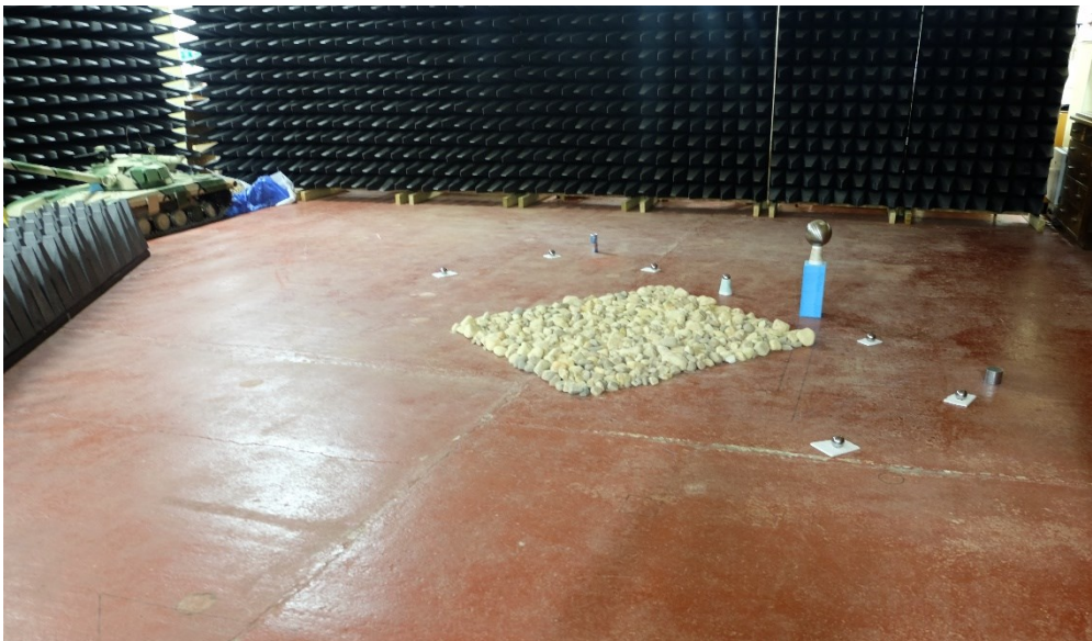
Figure 4.8 Image showing the stone rectangle within the laboratory environment. The spheres and top hat scatterers shown in Figure 4.5 are in the same locations.
