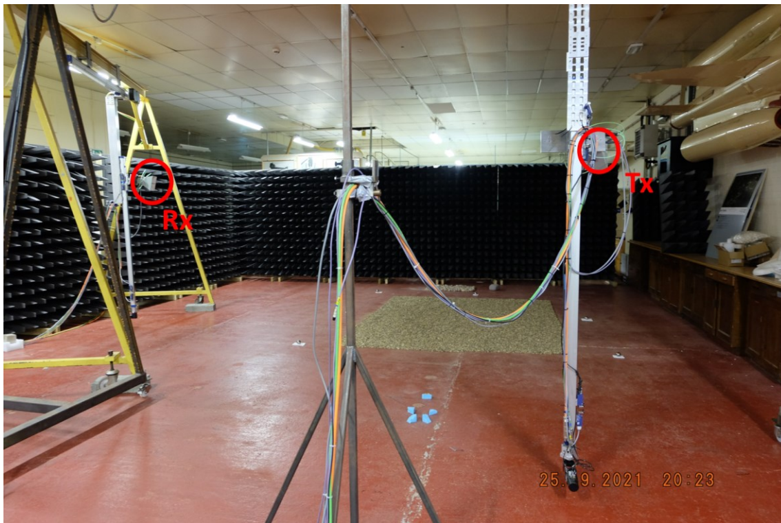
Figure 3.4. This image was taken from behind the transmitter (labelled Tx) and shows a bistatic configuration (receiver is labelled Rx). Two steel frames can also be seen (one brown and one yellow), these hold two motorised rails which allow the antenna horns to move within their two-dimensional apertures. The scene in the image consisted of a gravel rectangle, with metal spheres around to aid in image alignment and quality assurance.
