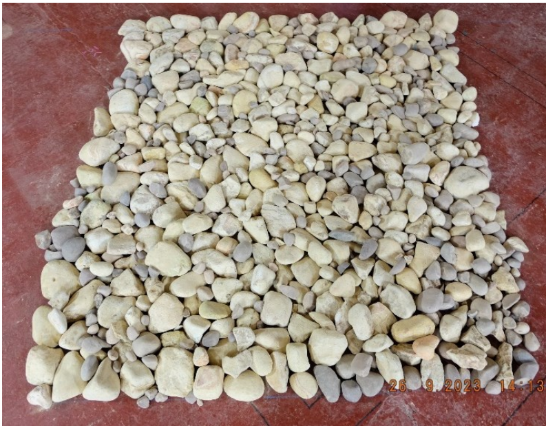
Figure 3.10 Image showing the stone rectangle. The alignment spheres and top hat scatterers are not shown in this image but were located in the same positions as in the gravel scene.
