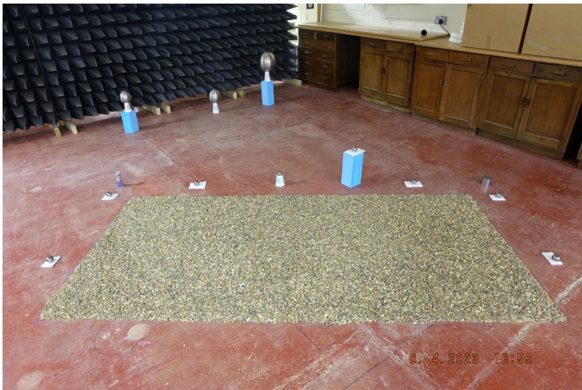
Figure 4.5 Image showing the gravel rectangle, together with spheres and top hat scatterers used to ensure image alignment.
