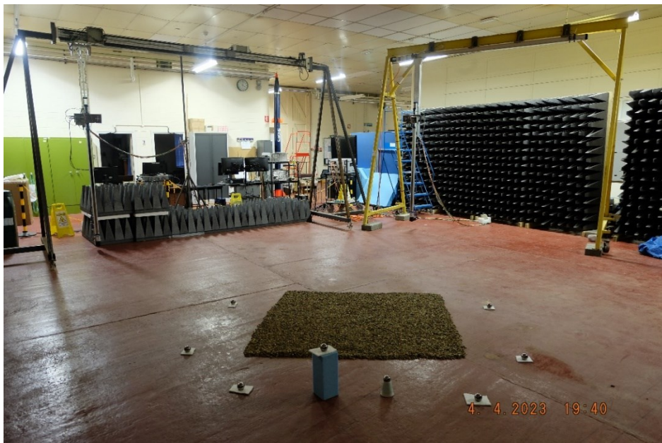
Figure 3.7 Photograph of a rotated rectangular gravel region which was aligned with the BEM.
