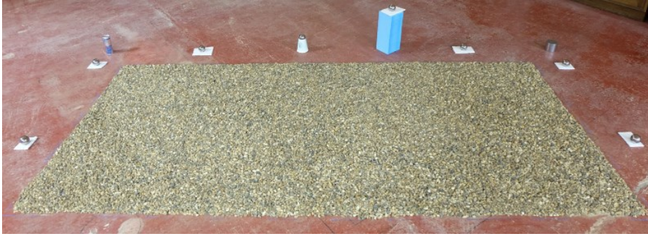
Figure 3.9 Image showing the gravel rectangle. The alignment spheres and top hat scatterers are shown.
