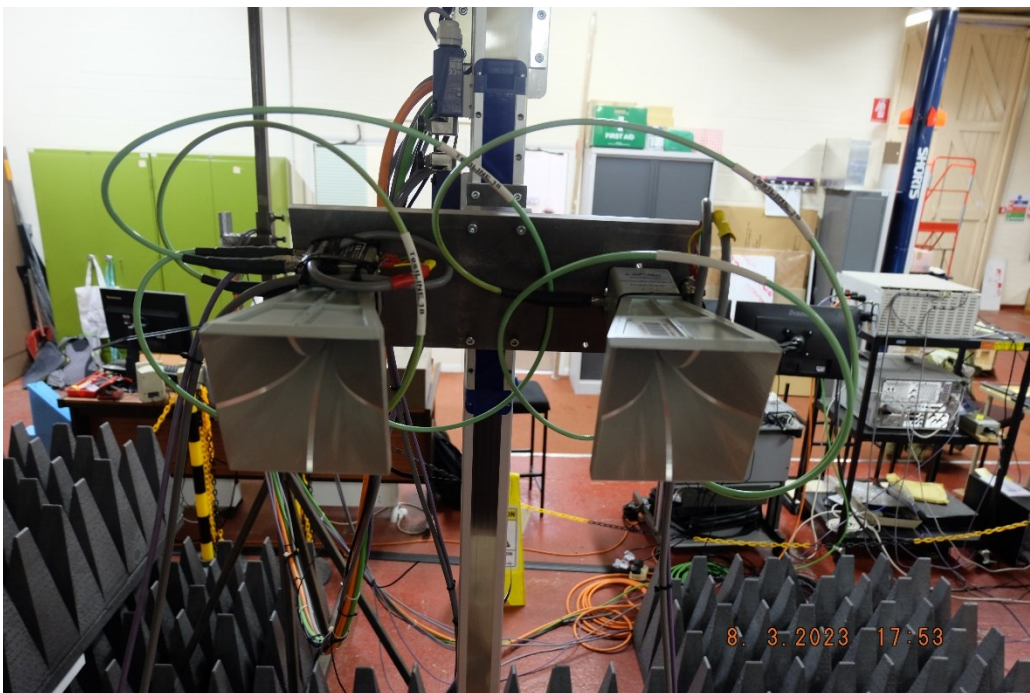
Figure 3.3 A-Info 2-18 GHz dual polarisation horn antennas setup in a monostatic configuration.
