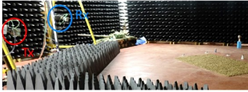
Figure 5 The GBSAR laboratory in a bistatic configuration. The transmitter is circled in red and labelled Tx; the receiver is circled in blue and labelled Rx.
