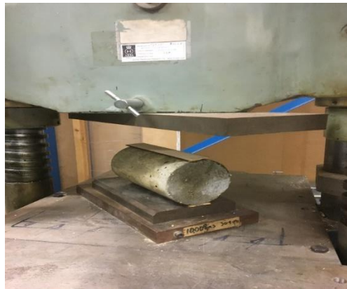
Figure 3-5 Mechanical tests of compressive, split tensile and flexural strengths.
