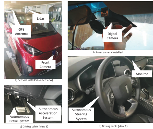
Fig. 7: Experimental setup: Sensors and Systems
