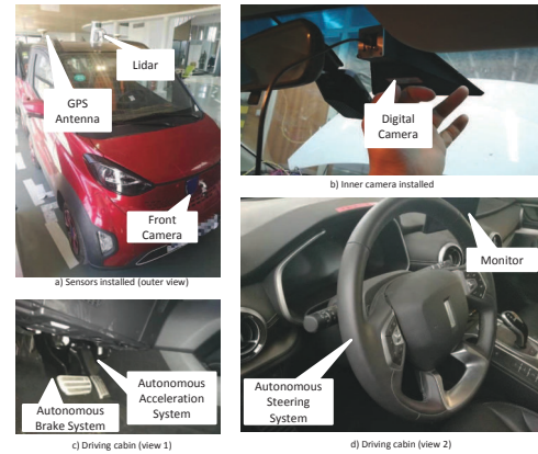
Fig. 7: Experimental setup: Sensors and Systems
