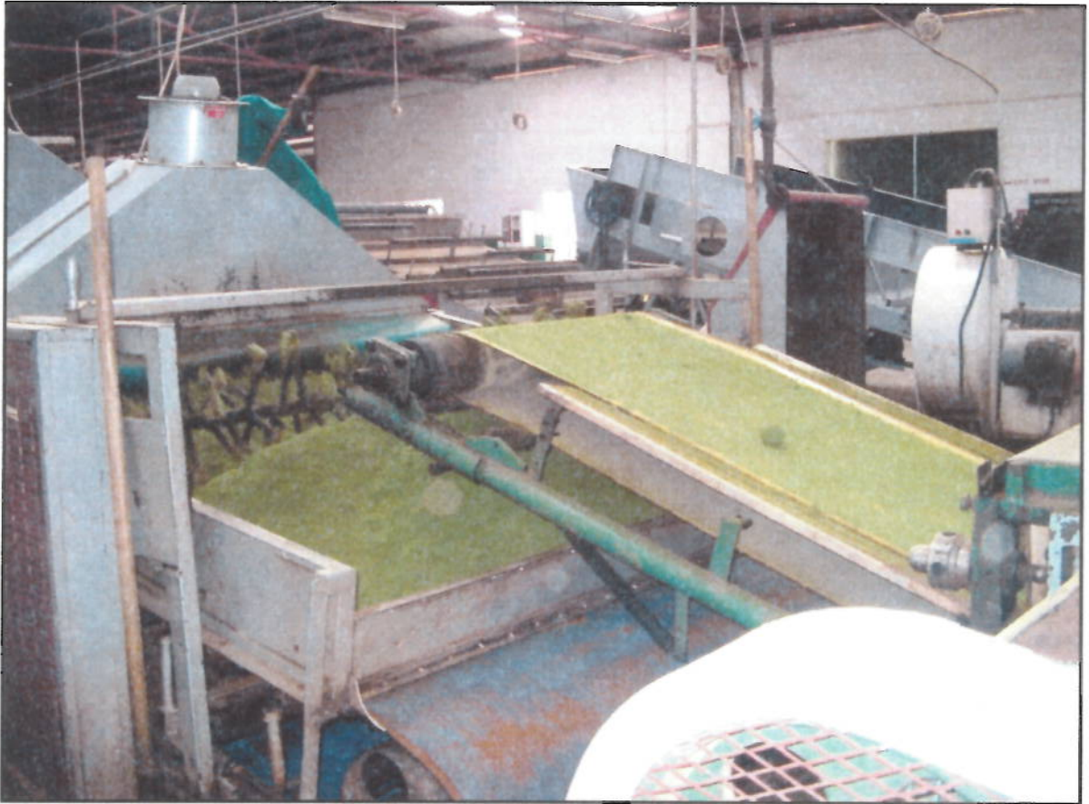
PLATE 6.3: Inside the tea processing factory, green leaf is being fermented ready for drying and sorting into market grades
