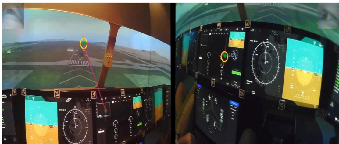
Fig. 5. PF's fixations switching between the centre of runway and cockpit displays demonstrated the attention distributions to maintain SA (left); PM's scanning patterns and fixations moving around AOIs to conduct cross-check with PF's operational procedures for instrument landing (right)
