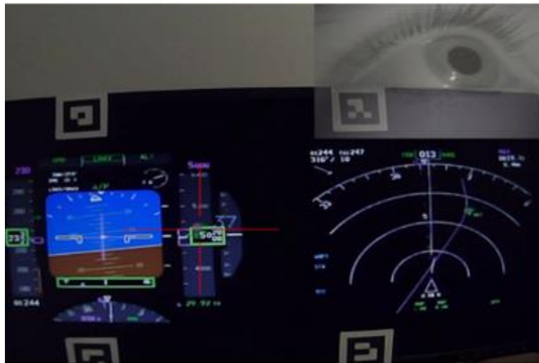
Fig. 1. Pilot's fixation at the altitude indicator (red-cross) and pupil dilation (right-hand side) on augmented design of PFD recorded by Pupil Eye Tracker (from [14])
