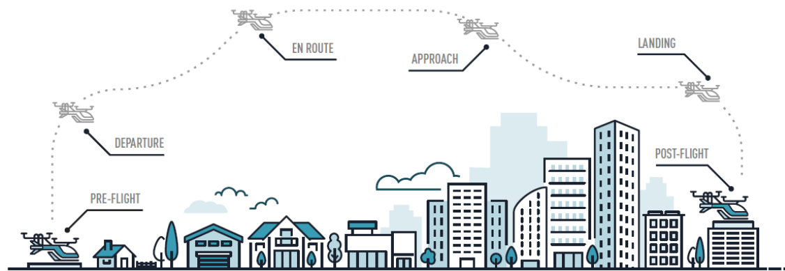
Figure 2-2. Phases of UAM flight. Source: (Airservices Australia & Embraer Business Innovation Center, 2020)
