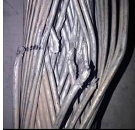
(b) Wire failure modes for V_i = 680 m/s
