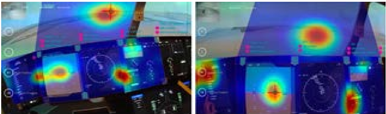
Figure 7 The heatmaps of PFs (left) demonstrated their visual attention mainly focused on the runway, PFD, and CUD; PMs (right) moving among four AOIs and the center of the runway while interacting with touchscreen controls on the instrument landing scenario
