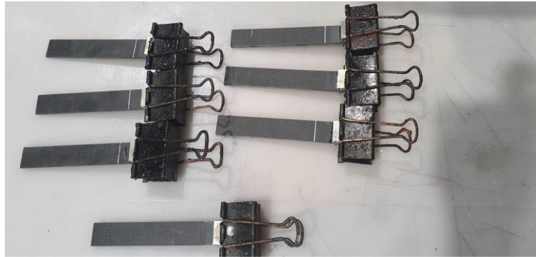
Figure 3.9. Mode 1 DCB specimens of DGEBA/4-APDS composite.
