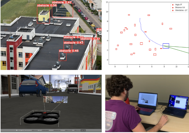
Fig. 6. Example results from the experimentation: (top-left) SLZ hazard detection, (top-right) autonomous navigation success to SLZ, (bottom-left) first person immersive view of landing, (bottom-right) pilot HITL measuring heart rate and controlling the eVTOL.
