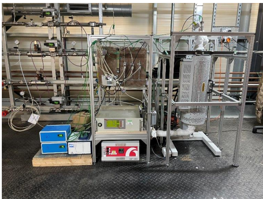
Figure 8-3 Constructed rig consisting of gas analysers on the left, mass flow controllers, a quartz reactor within a Carbolite furnace, joined via Swagelok fittings, and various other components.
