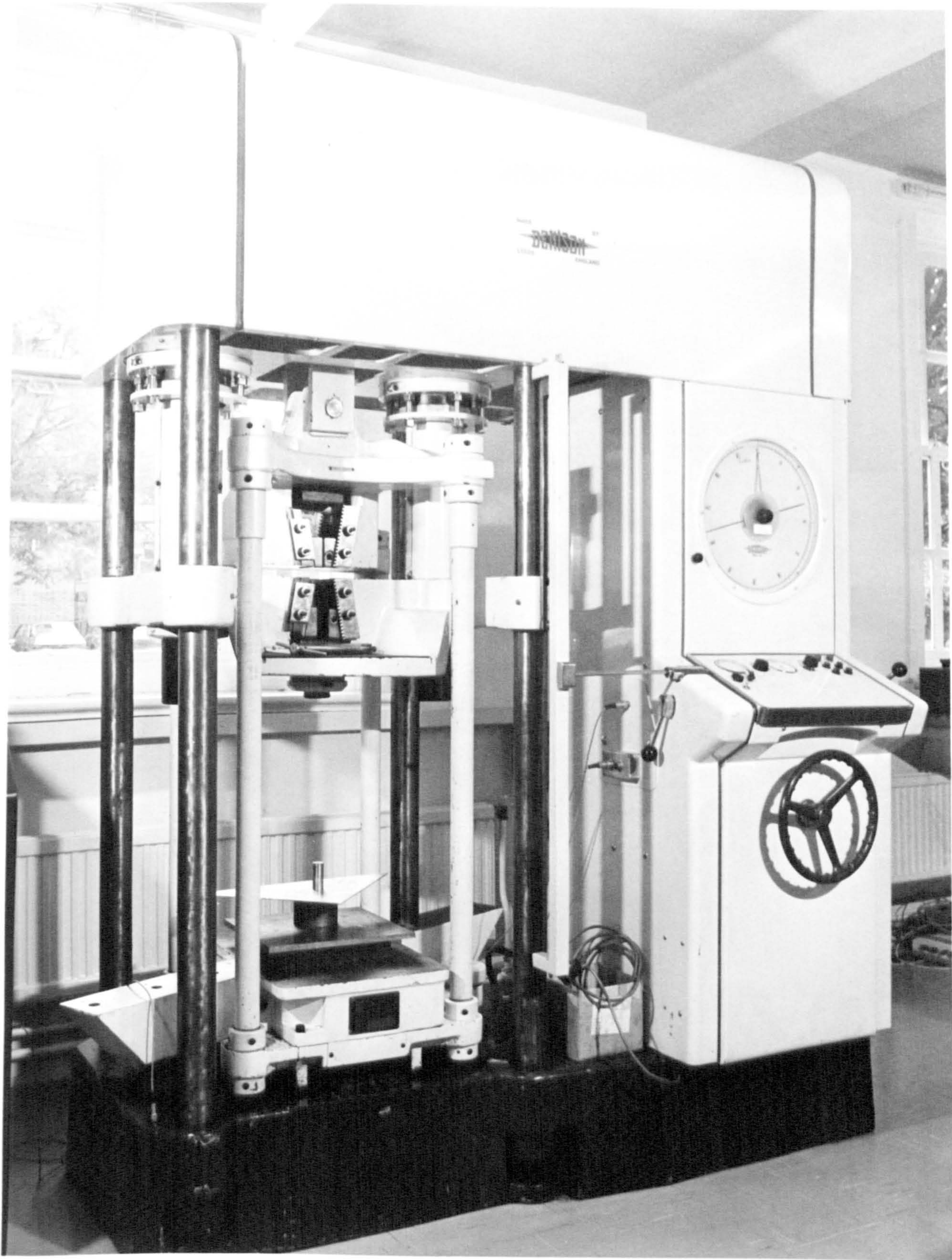
Plate 5.5 The Denison Compression machine used for pressing the specimen assemblies. Pressing capacity, 50 Tons.
