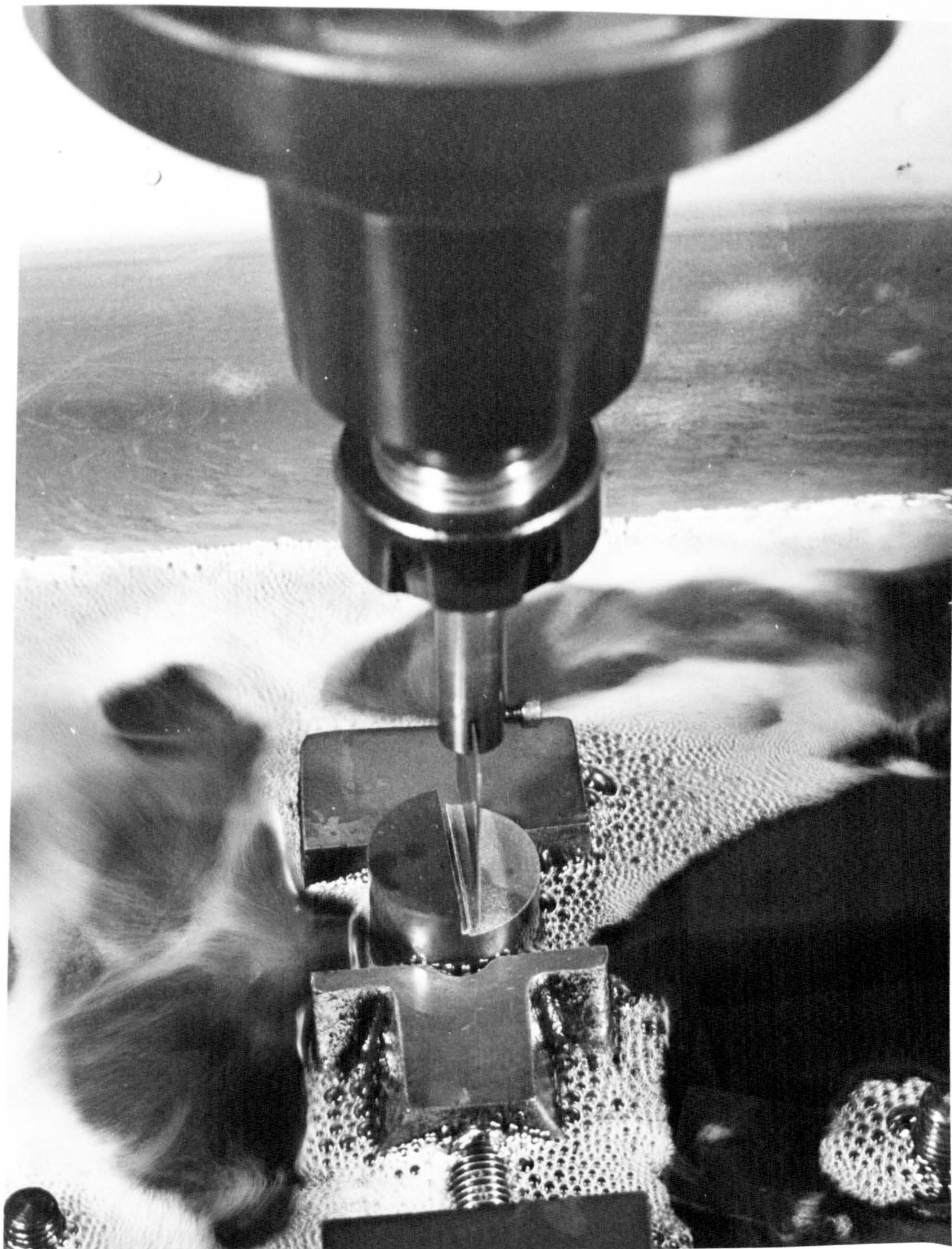
Plate 4.7 Spark erosion machine showing cutting operation of the oxidized specimen for microscopical film thickness measurements.
