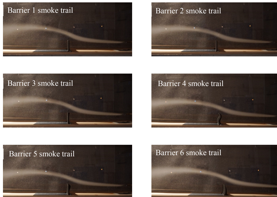
FIGURE 6. Wind tunnel results for all six barrier shapes
