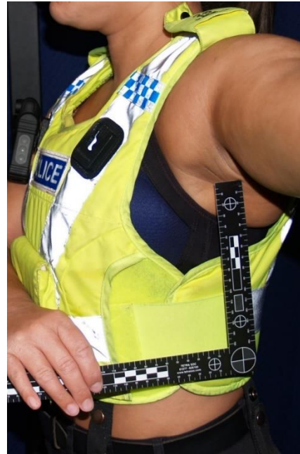
Figure 4-12 Example 2 – lack of overlap at side of body
