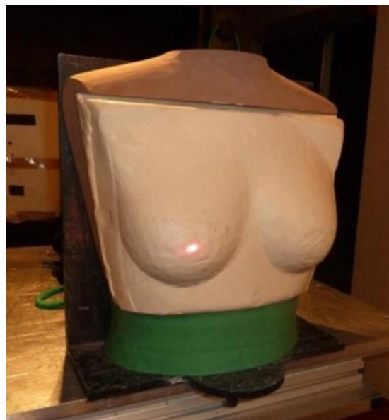
Figure 5-2 Example female test form as specified in Home Office Body Armour standard 2017 (image produced by author)
