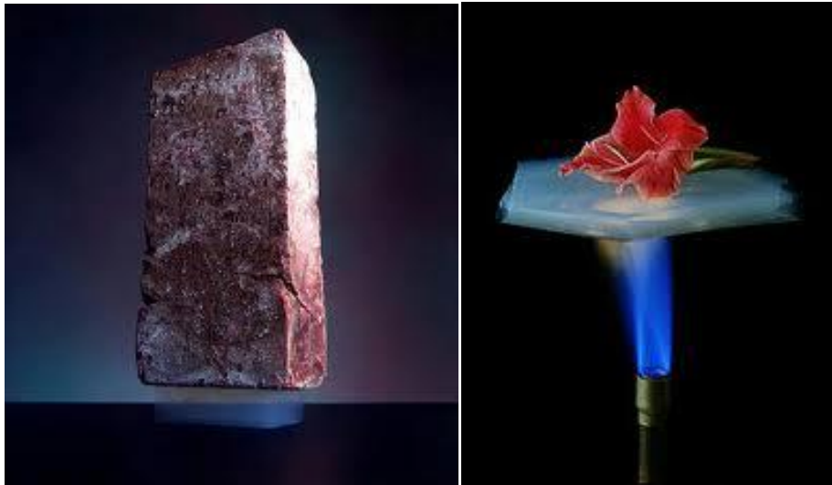
Figure 2-29 – Aerogel samples; the left picture is a 2.5 kg brick supported by a 2 g slice of Aerogel; the right picture is a flower being shielded from a naked blowtorch flame (NASA, 2004)
