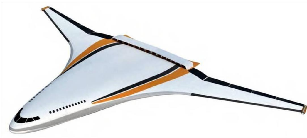
Figure 1-2 - NASA's N3-X Blended Wing Body (BWB) airframe concept (Armstrong et al , 2012)
