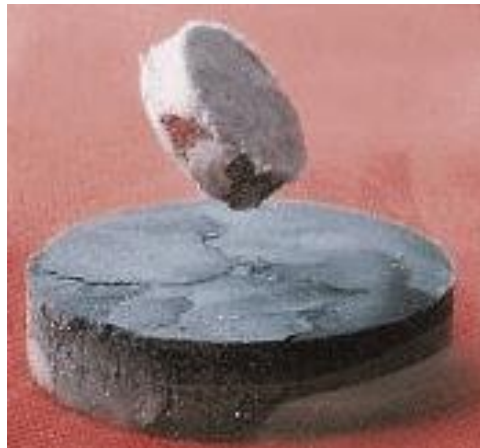
Figure 2-8 – Meissner effect of a HTS material (Warwick, 2000)
