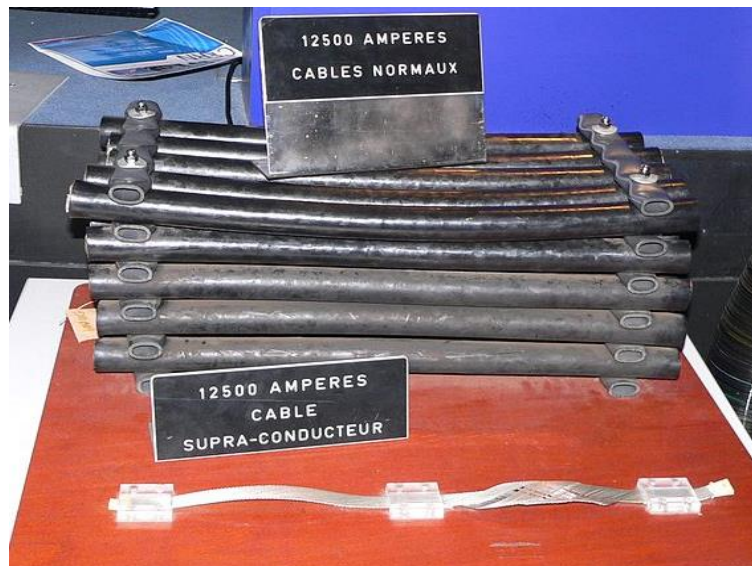
Figure 2-6 – Examples of equal current carrying capacity cables; conventional in the background, with superconducting in the foreground (CERN, 2006)
