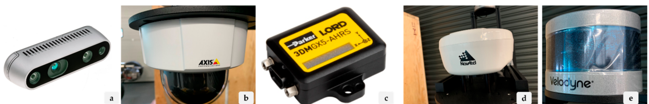
Figure 5. On-board sensors: (a) stereo depth camera; (b) environmental camera; (c) IMU; (d) RTK-GPS; (e) 3D Lidar.
