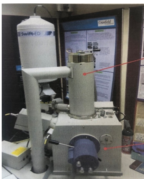
Figure 3-16 SEM used in experiments (Hitachi, SU5000)
