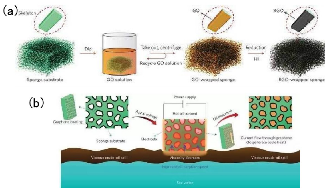
Figure 2-7 (a) Illustration of the production process of the graphene sponge; (b) Graphene foam adsorb high viscosity crude oil at sea [61]
