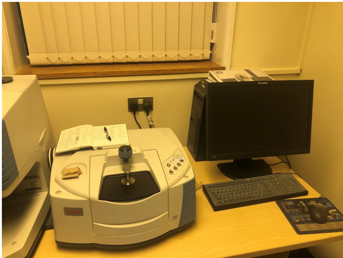
Figure 3-18 FTIR used in the experiment (Thermo Fisher, Nicolet iZ10)
