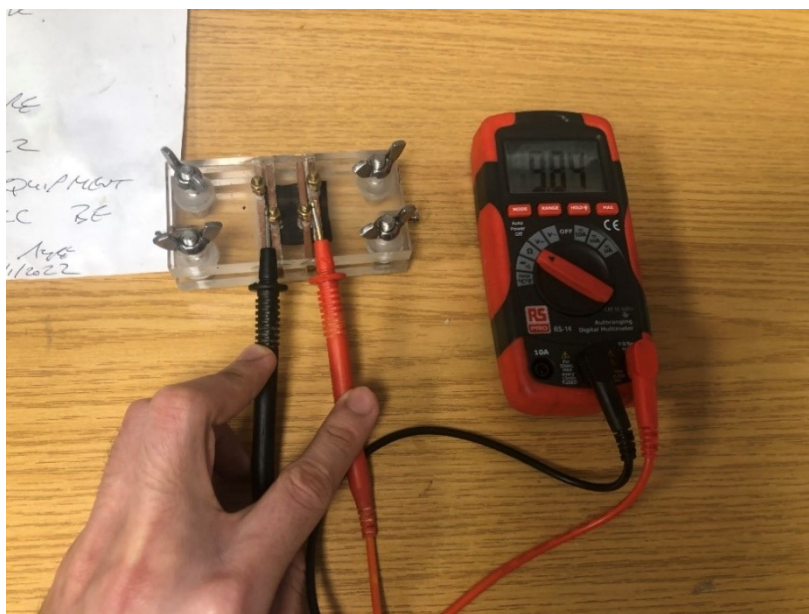
Figure 3-19 Photography of measuring resistance (RS PRO, RS-14)
