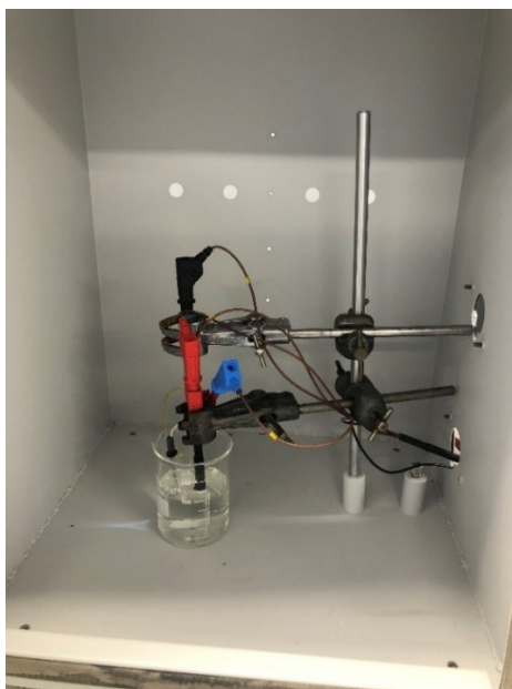
Figure 3-22 The three-electrode system used in the experiment (Cranfield)
