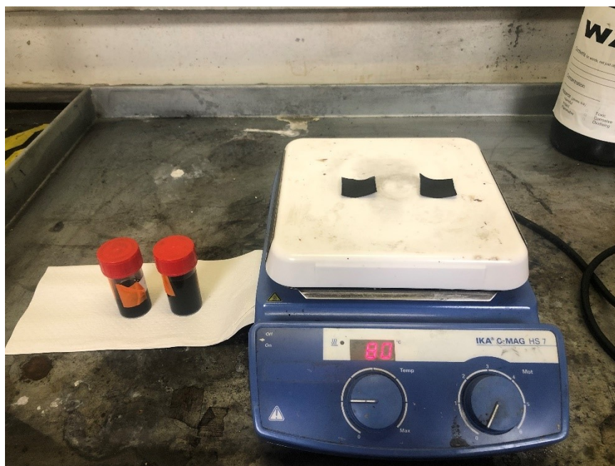
Figure 3-10 Drying process (IKA, C-MAG HS7)
