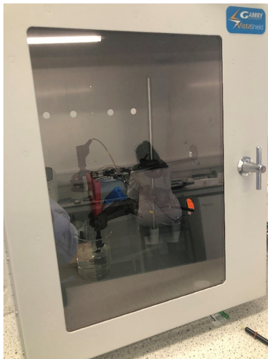
Figure 3-27 The electromagnetic shielding box used in the experiment (Cranfield)
