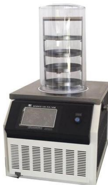
Figure 3-6 Freeze Dryer (Beijing Boyikang, Lab-50-1)
