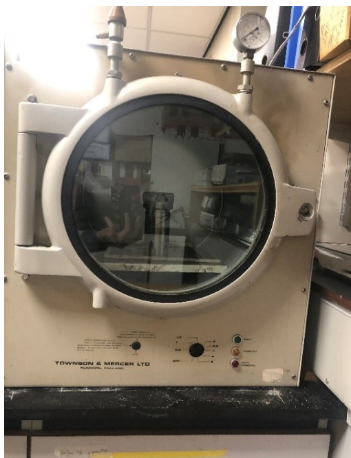
Figure 3-5 The oven used for heating in the experiment (Townson, F6010CN)
