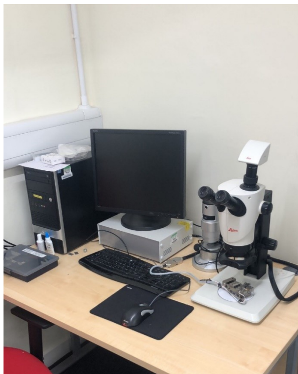
Figure 3-13 Optical microscope used in experiments (Leica, S9E)
