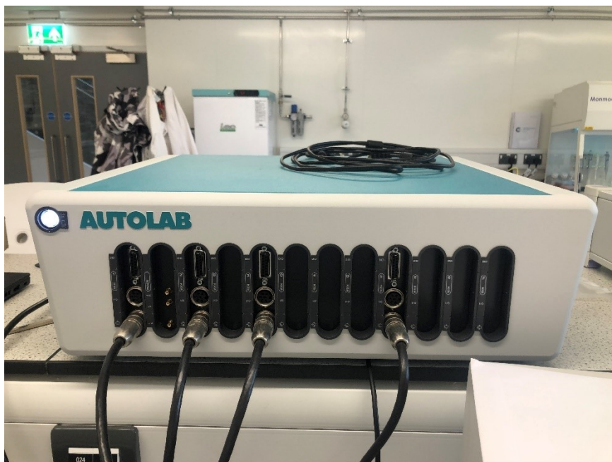
Figure 3-21 The electrochemical workstation used in the experiment (Autolab, 302N)
