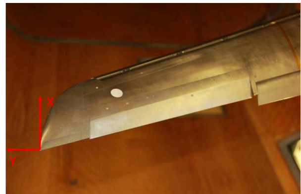
Fig 2: Photo of the aileron and trailing edge flap
