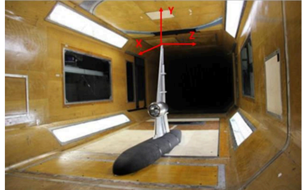
Fig 1: Wind tunnel model viewed from upstream
