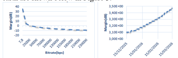
Figure 3: Link budgets from Mars to Earth using Mars Express and ESTRACK's [16].
