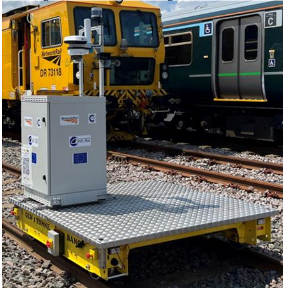
Fig.1 Autonomous Rail Trolley, equipped with LiDAR, GPS, Encoder and Camera
