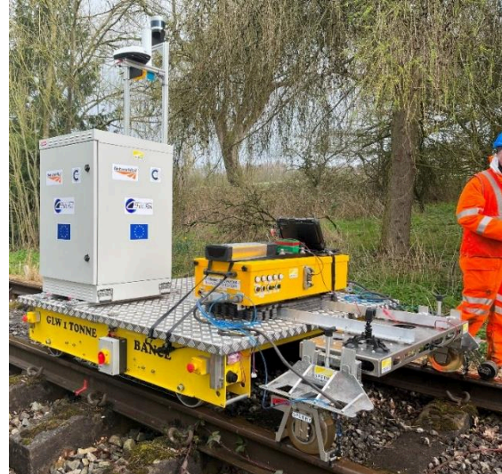
Fig.2 Integrated autonomous ultrasonic rail inspection system prototype
