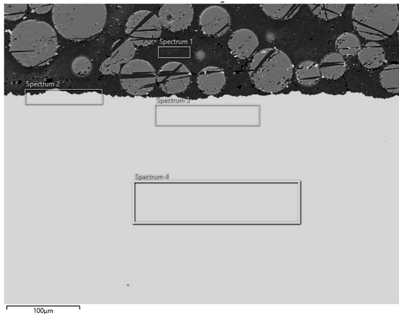
Figure 5-58 - SEM backscattered electron image of the exposed X100 3-point bent-beam sample in simulated saltwater solution with CO 2 at 25 °C stressed at 80 % Y.S. Data from the EDS spectra are reported in Figure 5-59.
