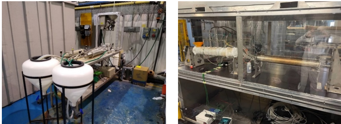
Figure 7-6 The test rigs showing the prototype components for the liquid processing side, left, and the solid fraction processing side, right. Photographed by project team.
