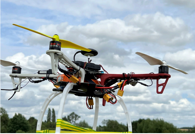
Fig. 4: Aerial Vehicle Platform for Experiment: DJI F450 Quadcopter
