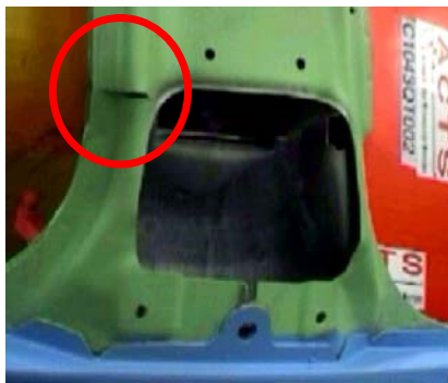
c) Test and simulation results showing critical location for failure
