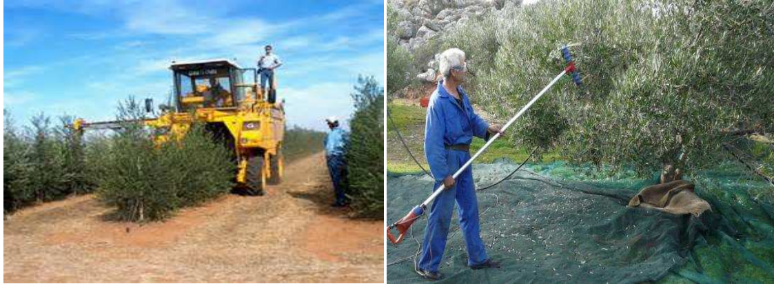
Figure1.10 (Left) Vehicle harvesting olives by vibration. (Right) Mechanical hand held beating harvester. Olives drop to the surrounding net and then gathered in sacks
