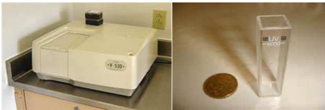
Figure 2.5 (Left) Jasco V-530, UV-VIS spectrophotometer used for the determination of UV (K indexes) absorbency. (Right) rectangular quartz cuvette of 1cm thickness used in spectroscopy of olive oil.
