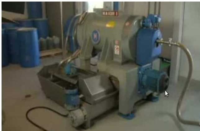
Figure 1.13 the separation of oil from the paste with decanter centrifugation
