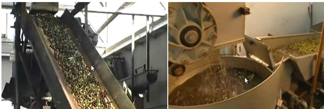
Figure 1.11 (Left) olives and other debris in the fruit elevator. (Right) olives are
