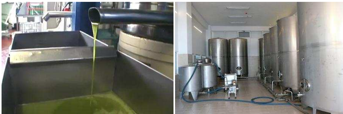
Figure 1.14 (Left) Olive oil after the separation ending in tanks of 1 m 3 . (Right) multiple tanks used for the storage of olive oil in bulk
