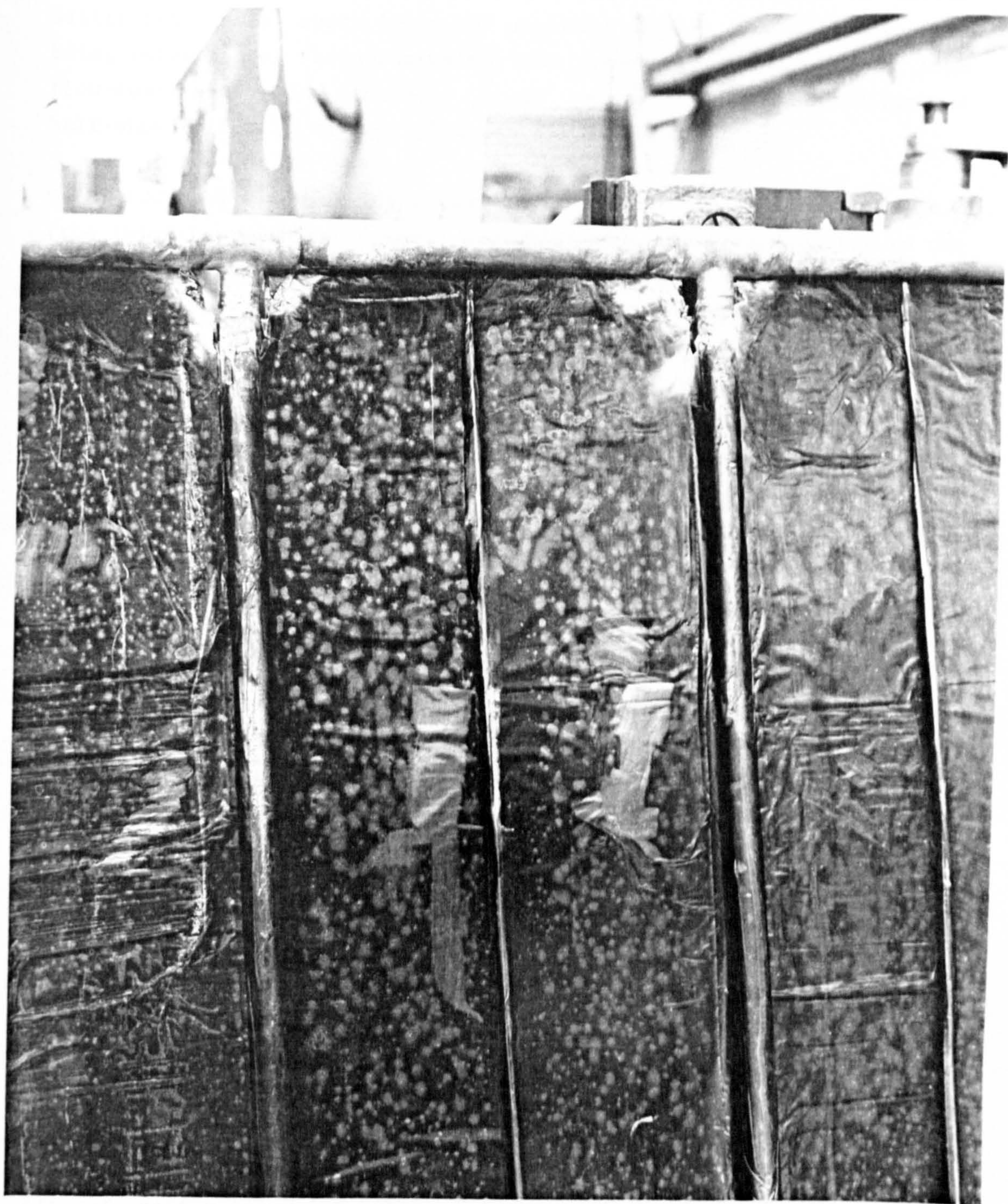
Figure 7.3.3 Degraded selective absorber surface
